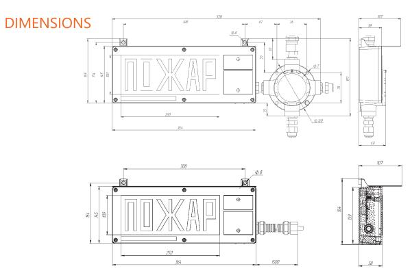
1Ex d mb [ib] IIC T4 Gb X
