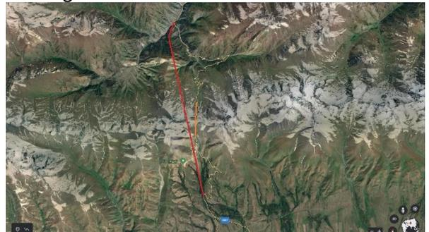
The alternative tunnel will avoid the serpentine at the entrance and exit of the existing tunnel and reduce the distance of 34 km to 11 km, reduce the time to pass the existing tunnel and serpentine from 2 hours to 11 minutes, and the spent fuel for trucks from 17 liters to 3.6 liters.
